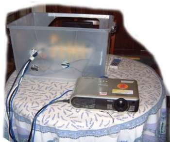
Fig 3. Showing the holes cut in the carry box for cable access and visibility.
