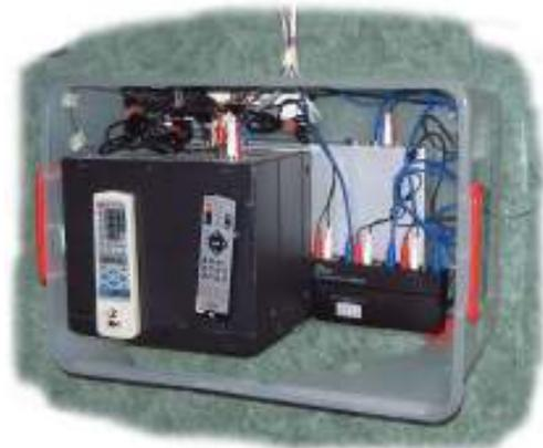
Fig 2. Fully pre-wired with all cables neatly(!) arranged, and only 5 leads leaving the package (taped together)
